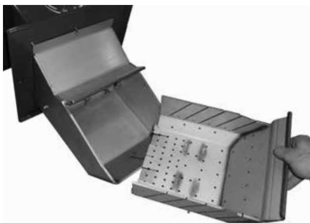
Removable combustion chamber of the burner with air supply openings - must be checked regularly
