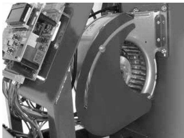
Fan of the burner with an air flap. By opening the air flap you will reduce the length of the flame
