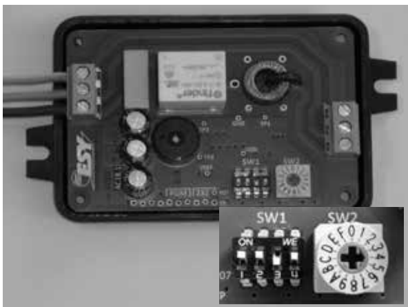
Module AD01 – opened for setting it up
