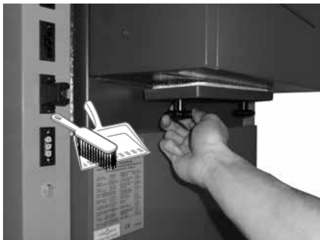
Sample cleaning of the smoke duct at the back side of the boiler
